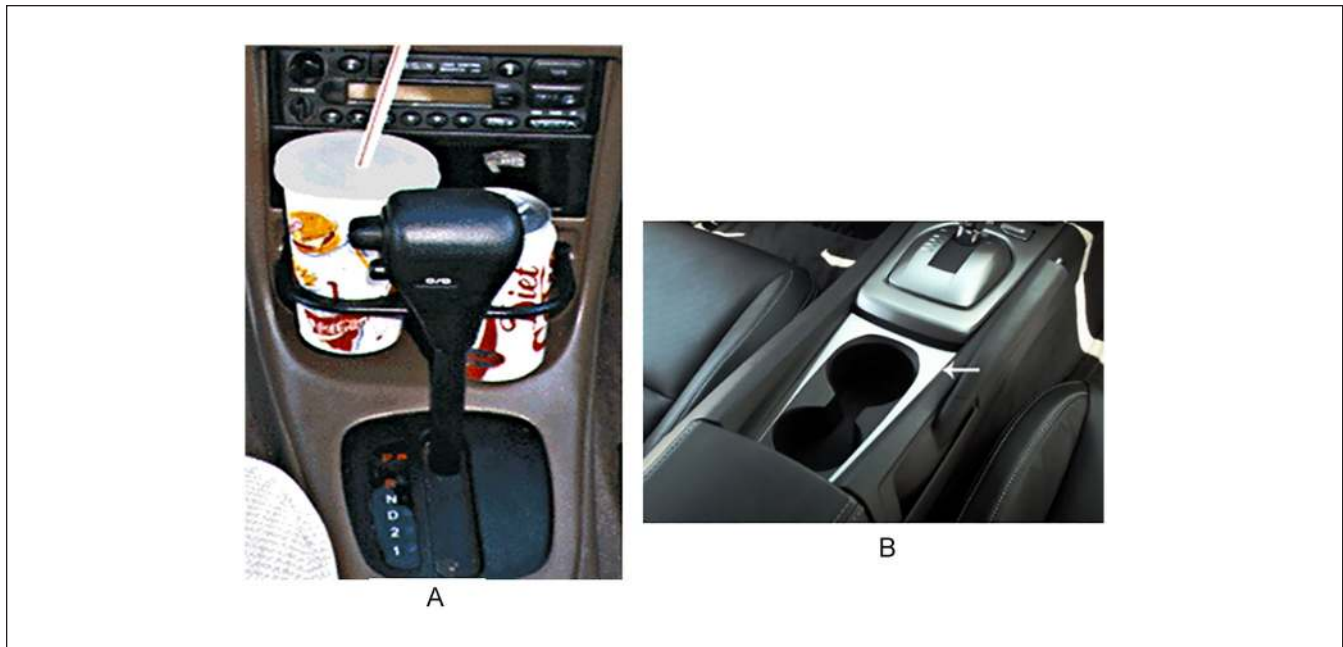
Figure 5. Bad design of cup holder (A) and good redesign (B) as an ethical solution.
