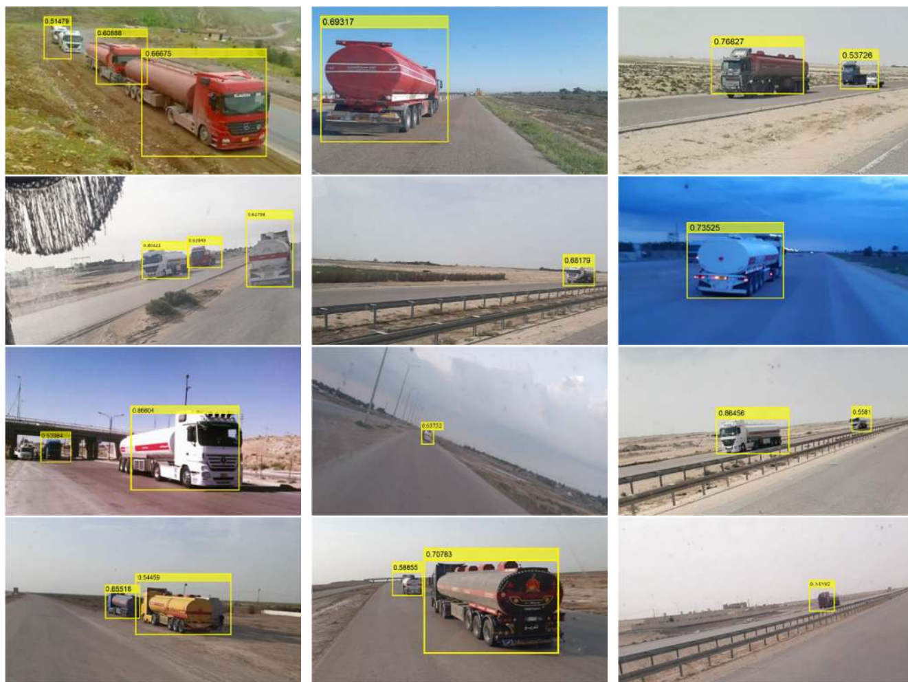
FIGURE 6. Selected examples of fuel truck detection results on the fuel truck dataset using the proposed OYOLOv2_FTD. Each output box is associated with the score, and the detected frame rate is displayed in the upper-left corner.
