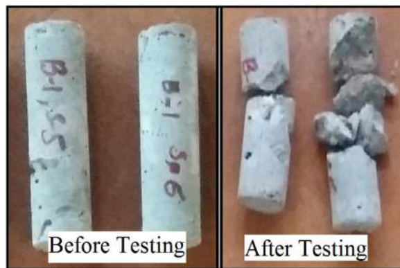
Fig. 7. Concrete Pencil Specimens before and after testing.
