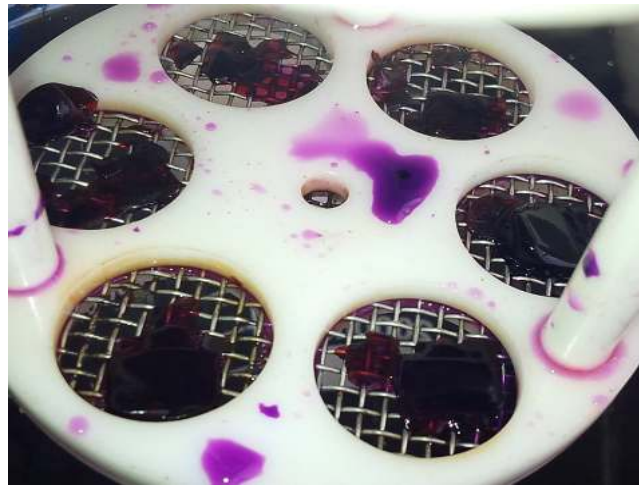
Figure 6: The disintegration apparatus basket at 60 min showing the remains of Capsule 6 type on the mesh when tested in SIF.
