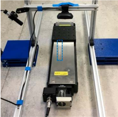
Figure 5: 2D scanning system with a linear actuator; 2D map is obtained from attaching 1D profiles, where the laser line is highlighted in a dashed rectangle.
