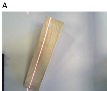
Figure 6: The experimental results for a simple surface (woody wedge), including (A) test image with projected laser line, and (B) obtained levelness H(x) from the wedge sample.
