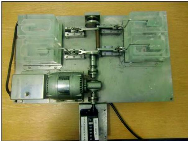
FIGURE 1: Toothbrush-simulating machine.
