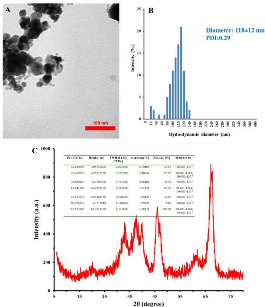
Fig. 1 TEM image (A), DLS histogram (B), and XRD pattern (C) of synthesized  $\text{Al}_2\text{O}_3$  NPs. The inset shows the XRD data.
