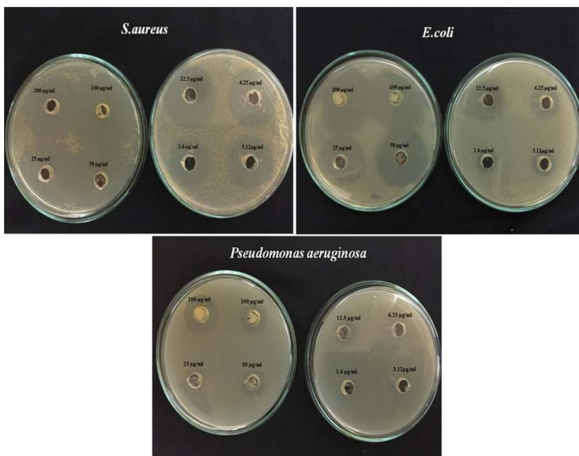
**Fig. 7** Visible zone produced by varying concentrations (200–3.12 µg/ml) of Al<sub>2</sub>O<sub>3</sub> NPs against *S. aureus*, *E. coli* and *P. aeruginosa*.
