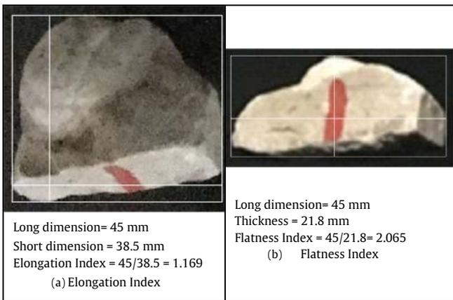
Fig. 4. Sample calculation of elongation and flatness indices.
