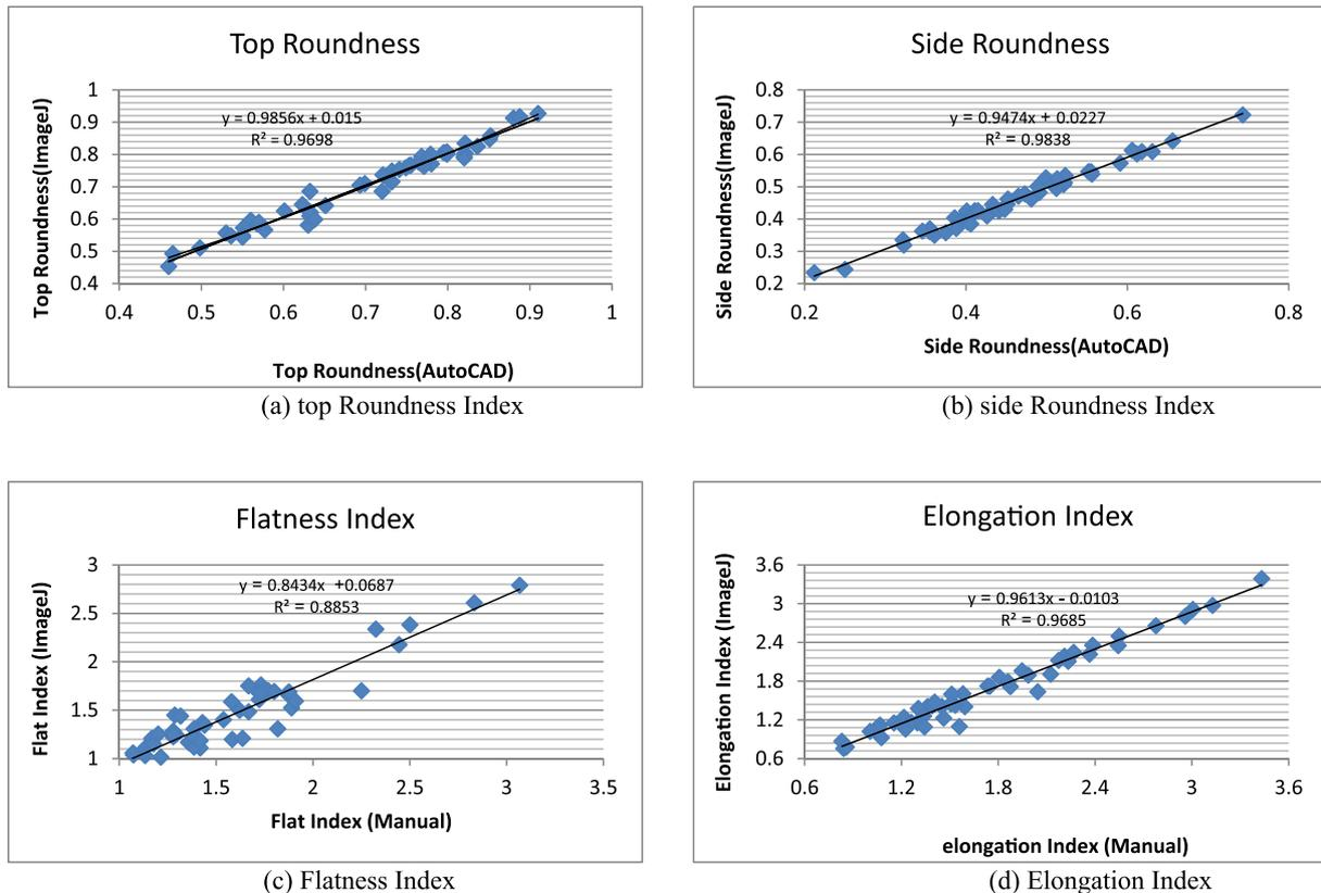
Fig. 13. Relationships between the coarse aggregate shape properties from AutoCAD (and caliper) and from ImageJ.
