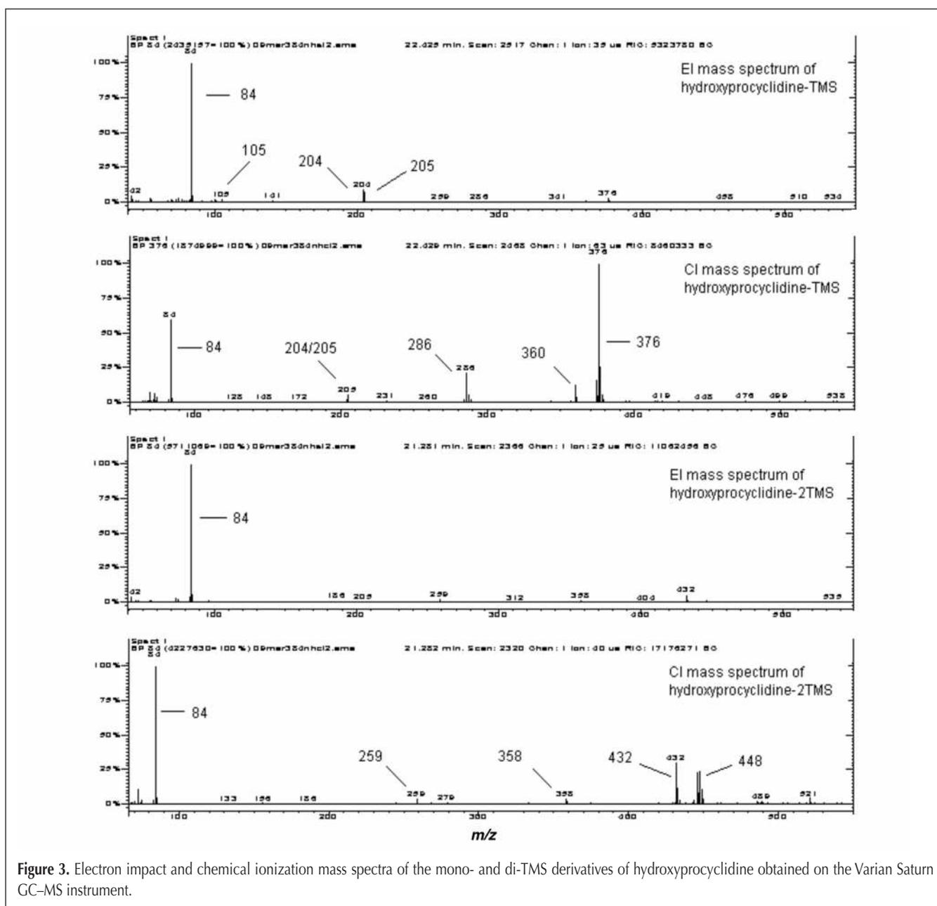
Figure 3. Electron impact and chemical ionization mass spectra of the mono- and di-TMS derivatives of hydroxyprocyclidine obtained on the Varian Saturn GC-MS instrument.
