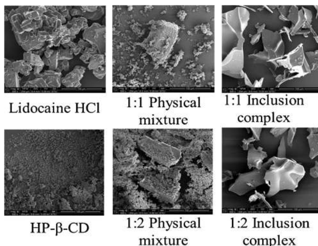
Fig. 7. Scanning electron microscopy images of lidocaine HCl, HP- \beta -CD, 1:1 and 1:2 lidocaine HCl/HP- \beta -CD physical mixtures, and 1:1 and 1:2 lidocaine HCl/HP- \beta -CD inclusion complexes, \times 500 magnification, \text{bar}=100 \mu\text{m} .
