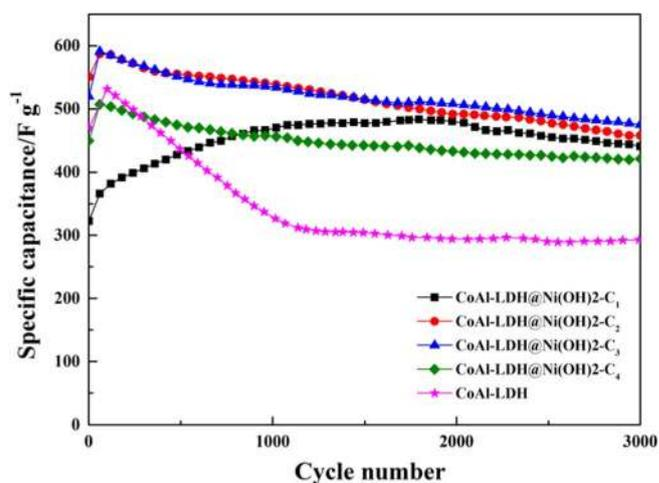
**Figure 11.** Cycle stability of the CoAl-LDH@Ni(OH)<sub>2</sub> electrodes and pure Co-Al-LDH electrode at 30 A g<sup>-1</sup> for 3000 cycles.
