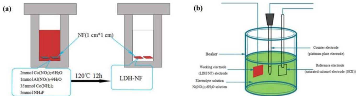
**Figure 1.** (a) Schematic illustrations of synthesis process for CoAl-LDH composites and (b) CoAl-LDH@Ni(OH)<sub>2</sub> composites.
