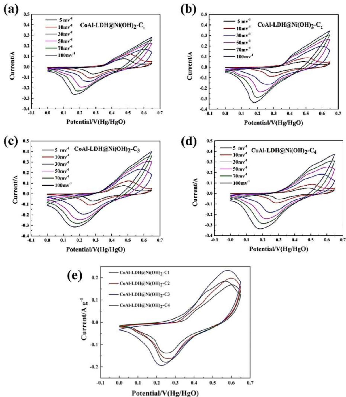
**Figure 8.** (a-d) Cyclic voltammograms of CoAl-LDH@Ni(OH)<sub>2</sub> were obtained by electrodeposition different number of cycles in 6-M KOH aqueous solution, respectively and (e) in 6-M KOH aqueous solution at 30 mV.
