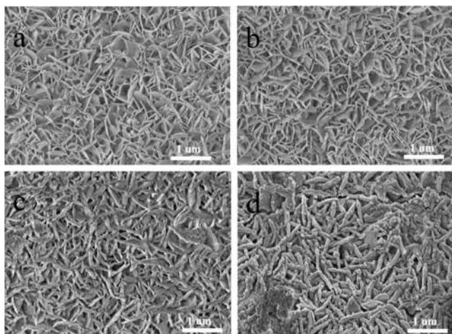
**Figure 5.** The SEM images (a), (b), (c), (d) of CoAl-LDH@Ni(OH)<sub>2</sub> were obtained by electrodeposition at 4 cycles, 6 cycles, 8 cycles, and 10 cycles, respectively.
