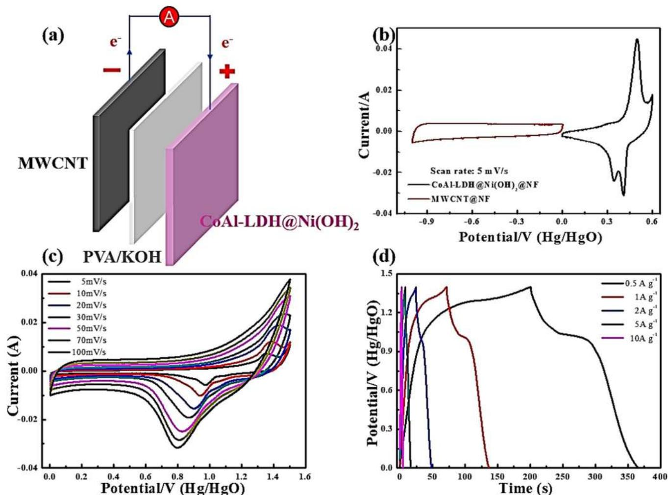
**Figure 12.** (a) Schematic illustration of the SASC device, (b) CV curves of MWCNT and CoAl-LDH@Ni(OH)<sub>2</sub> electrode in three-electrode system at scan rate of 5 mV<sup>-1</sup>, (c) CV curves of SASC device at different scan rates, (d) Charge-discharge curves at different current densities.
