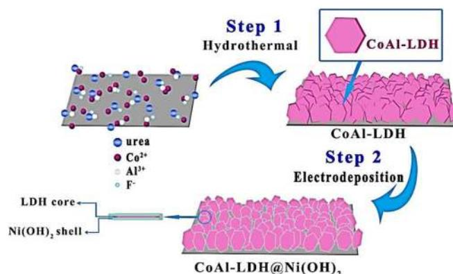
**Figure 2.** Schematic and SEM illustration of the two steps synthesis of hierarchical CoAl-LDH@Ni(OH)<sub>2</sub> electrode.
