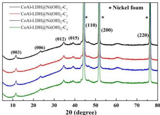
Figure 3. XRD patterns of CoAl-LDH@Ni(OH)<sub>2</sub>.
