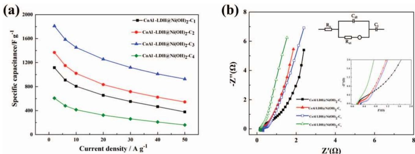
**Figure 10.** (a) Specific capacitance of the CoAl-LDH@Ni(OH)<sub>2</sub> electrodes with different electrodeposited cycles, and (b) Nyquist plots of the CoAl-LDH@Ni(OH)<sub>2</sub> electrodes.
