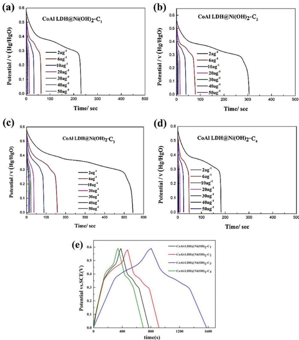
**Figure 9.** (a-d) Charge/discharge curves CoAl-LDH@Ni(OH)<sub>2</sub>-C<sub>1</sub>, CoAl-LDH@Ni(OH)<sub>2</sub>-C<sub>2</sub>, CoAl-LDH@Ni(OH)<sub>2</sub>-C<sub>3</sub>, and CoAl-LDH @Ni(OH)<sub>2</sub>-C<sub>4</sub> at current densities of 2, 6, 10, 20, 30, 40, and 50 A g<sup>-1</sup> in 6-M KOH aqueous solution. (e) Charge/discharge curves of the comparison of the CoAl-LDH@Ni(OH)<sub>2</sub> electrodes with different electrodeposited cycles at 2 A g<sup>-1</sup>.
