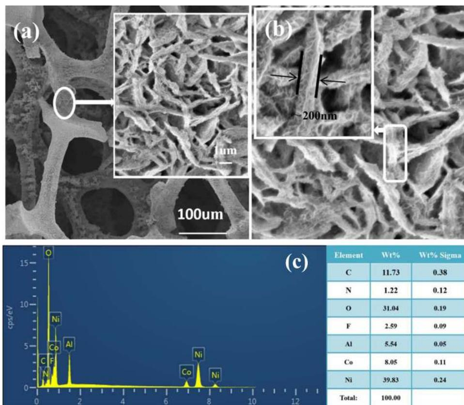
**Figure 6.** (a) and (b) The SEM images of CoAl-LDH@Ni(OH)<sub>2</sub> were obtained by electrodeposition at 8 cycles at different magnification and (c) Quantitative analysis of EDS in large scope.
