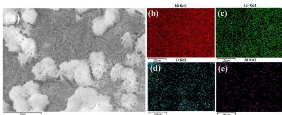
**Figure 7.** (a) SEM image of the CoAl-LDH@Ni(OH)<sub>2</sub>-C<sub>3</sub> composite, the EDS mapping of (b) Ni, (c) Co, (d) O, and (e) Al.
