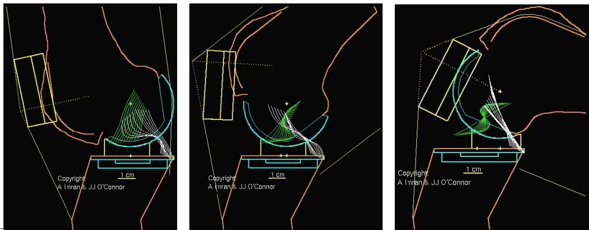
Fig. 2. The model knee shown at 0°, 60° and 120° flexion.
