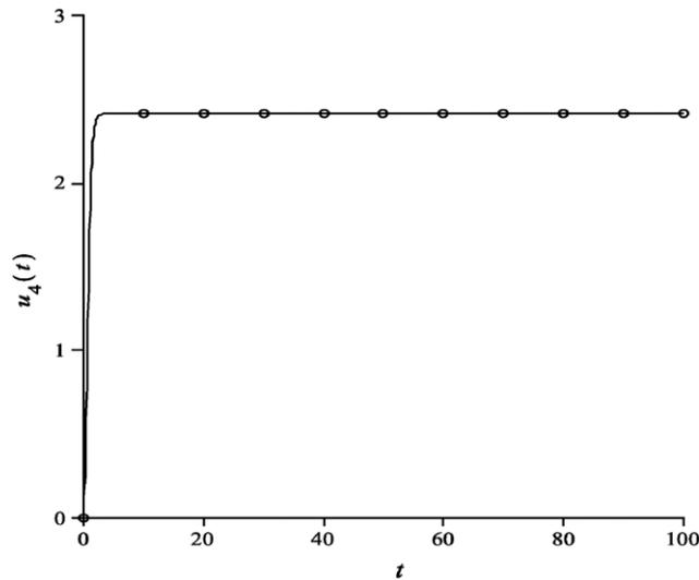
**Fig. 1.** Approximate solution for Example 4.1 using the fourth-order PTV algorithm when  $\Delta t = 0.1$ , where the fourth-order PTV solution is given by the circle symbols and the exact solution is given by the solid line.
