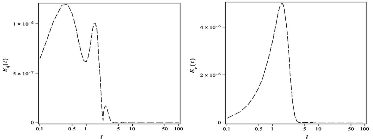
**Fig. 4.** The absolute errors of the fourth-order PTV solution (left) when  $\Delta t = 0.1$  ( $E_4(t) = |u_{RK78}(t) - u_4(t)|$ ) and the numerical RK4 solution (right) when  $h = 0.1$  ( $E_r(t) = |u_{RK78}(t) - u_{RK4}(t)|$ ) for Example 4.2.
